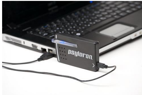
Psyleron random number generator, attached to a laptop PC.
